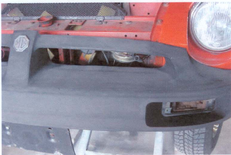
Bumper after cleaning with wax & grease remover and initial sanding
