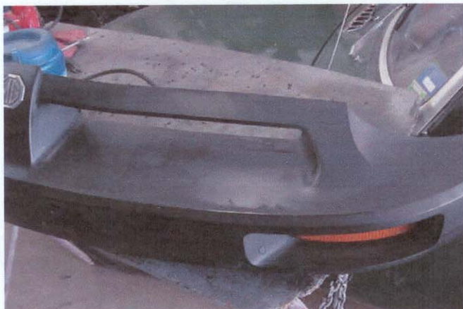
Before repairs. Notice the dull, crazed finish. Home restorers should remove bumpers first
